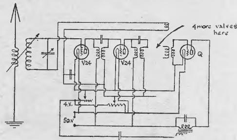
Fig. 4—Marconi 7-valve Amplifier, Type 55A.
