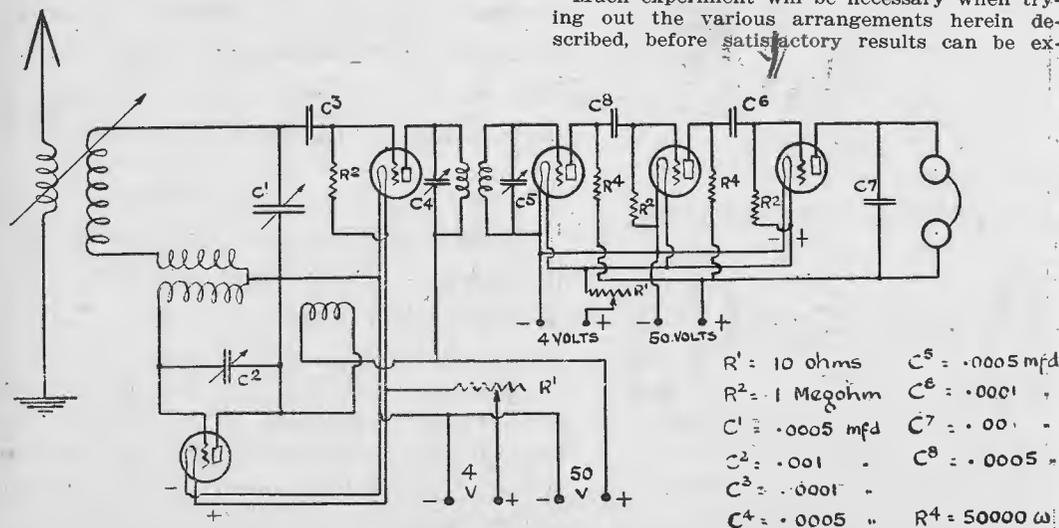
Fig. 1—Resistance-coupled Amplifier with Separate Heterodyne.
