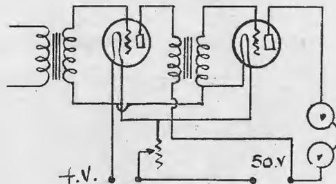
Fig. 3—Low-frequency Amplifier.
