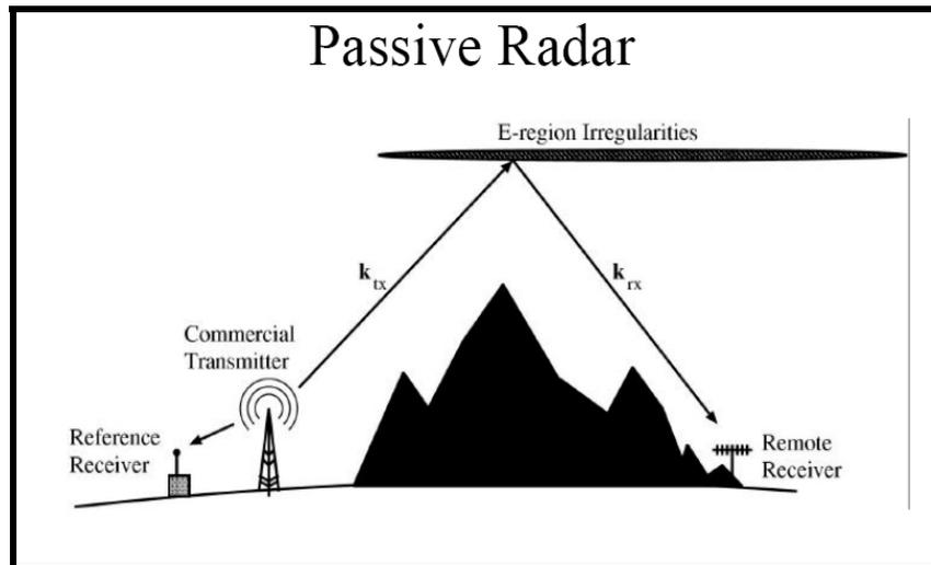
*Figure 5: Schematic of typical passive, bi-static radar system. ( Note Reference Receiver on left,, necessary for registering original transmitted signal.). (Source: Prof. John Sahr, [jdsahr@u.washington.edu](mailto:jdsahr@u.washington.edu); <http://rrsl.ee.washington.edu/>)*
