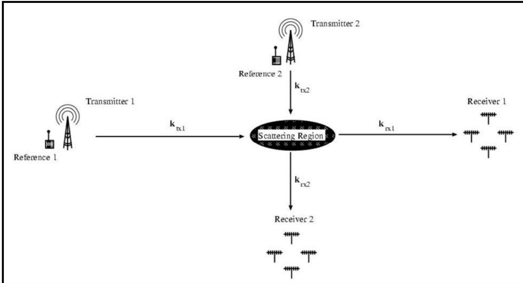
**Figure 6:** A multi-static, passive array, employing two transmitters, and two sets of receivers, each with four antennas. (Source: Prof. John Sahr, [jdsahr@u.washington.edu](mailto:jdsahr@u.washington.edu); <http://rrsl.ee.washington.edu/>)
