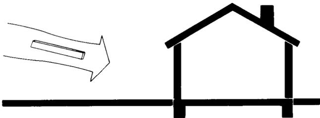
**Figure 3. Impact forces created by missiles.**
