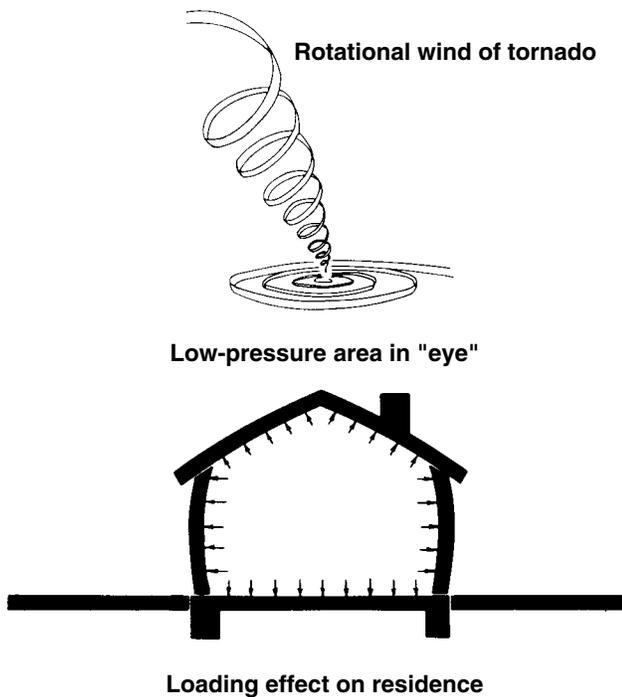
**Figure 2. Pressure forces created by sudden pressure drop.**
