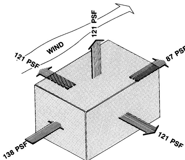
Figure 1. Pressure forces created by 240 mph wind.
