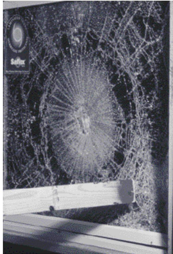
An impact-resistant window system after being hit by a large missile. Though the glass has shattered, it remains intact, thus preventing wind and rain from entering the building.
