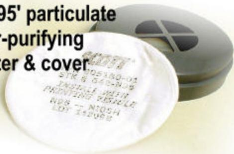
R-series filters are oil-resistant; and P-series filters are oil-proof (see figure above right). N-series filters can only be used for protection from non-oil aerosols because certain compounds can degrade their efficiency over time. So, do not use the N-series filters when oil may be present. Each of the three grades of filters has three levels of filter efficiency (95%, 99%, and 99.97%); higher efficiency means lower filter leakage.
