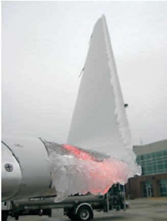
Accumulation of ice on aircraft is one of the most significant hazards to the safe and efficient operation of aircraft as it can reduce aircraft performance in a number of ways. Aircraft flying through cloud in sub-freezing temperatures are likely to experience some degree of icing.
