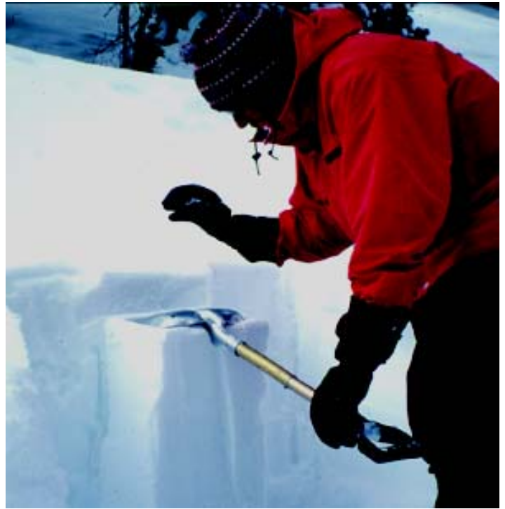
A compression test on an isolated column is one of several snow pit tests that can help assess snowpack stability
