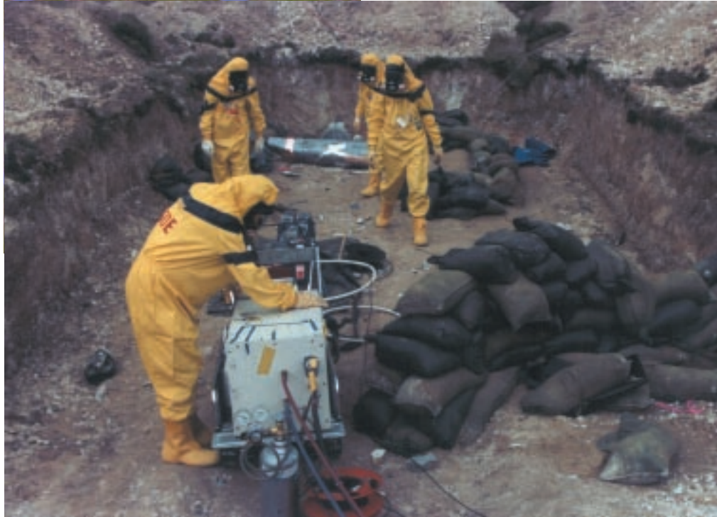
Specialized techniques, such as radiography, are used to examine the weapon's internal structure.
